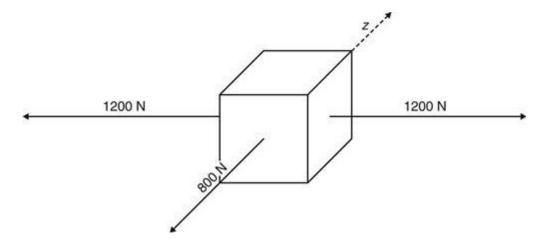
If the crate is to remain stationary, what amount of force must be applied for *z*?
