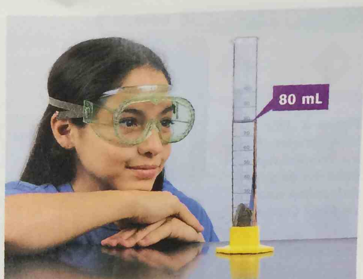
Figure 3 Adding the rock changes the water level from 70 mL to 80 mL. So, the rock displaces 10 mL of water. Because 1 \text{ mL} = 1 \text{ cm}^3 , the volume of the rock is 10 \text{ cm}^3 .
